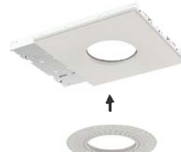
1. Fasten mud frame to ceiling.
